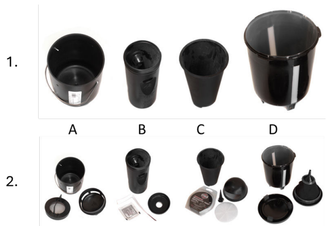
Figure 2: 1) The main trap body (the external bucket); 2) all the components of the traps. A) Trap-N-Kill Mosquito Trap; B) SKEET-O-TRAP; C) STUCK® OUTDOOR Mosquito Trap; D) New experimental ovitrap; 2) Internal parts of the traps (in the same order).
