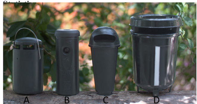
Figure 1. Traps tested during the study: A) Trap-N-Kill Mosquito Trap, B) SKEET-O-TRAP, C) STUCK® OUTDOOR Mosquito Trap, D) New experimental ovitrap.
