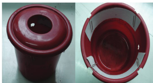
Figure 3. Sticky Ovitrap showing external and internal parts of the trap. The sticky paper is attached above the interior water line.
