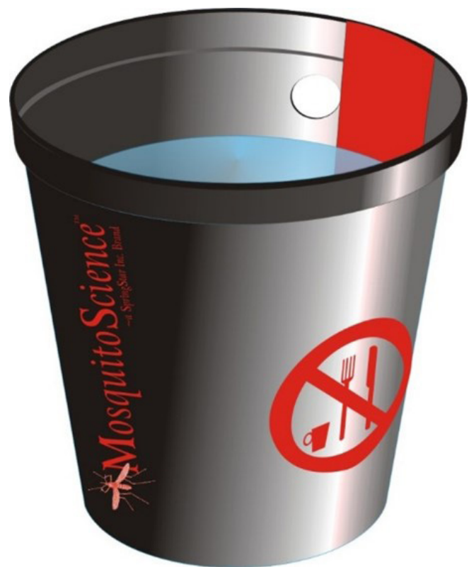
Figure 2. The Zeichner Lethal Ovitrap, a black plastic cup with a red strip of insecticide-treated oviposition paper attached. Overflow hole maintains water level.
